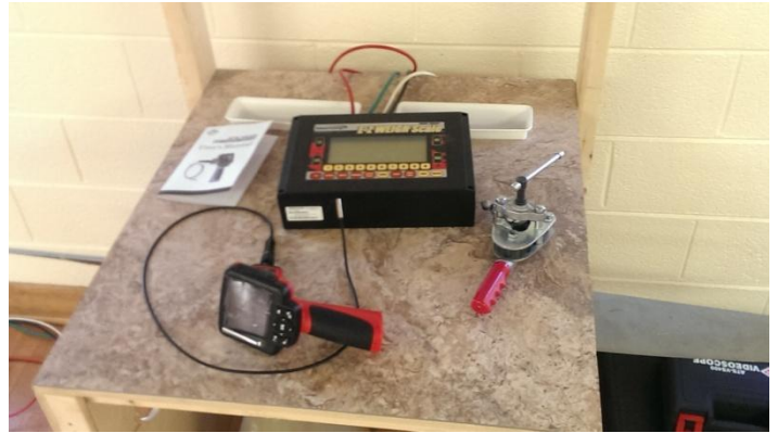
From the Tool Crib: Borescope camera, controller and readout for scales, and flaring tool.
